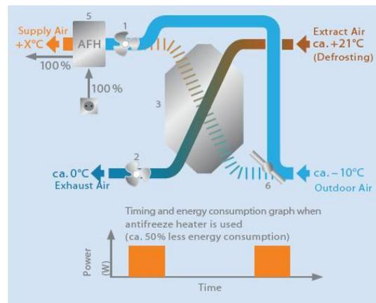
Thanks to the new smart frost protection facility the heater works only when it is needed and therefore consumes much less energy. This way the unit fully benefits from the heater with less individual pulses but longer running cycles.
