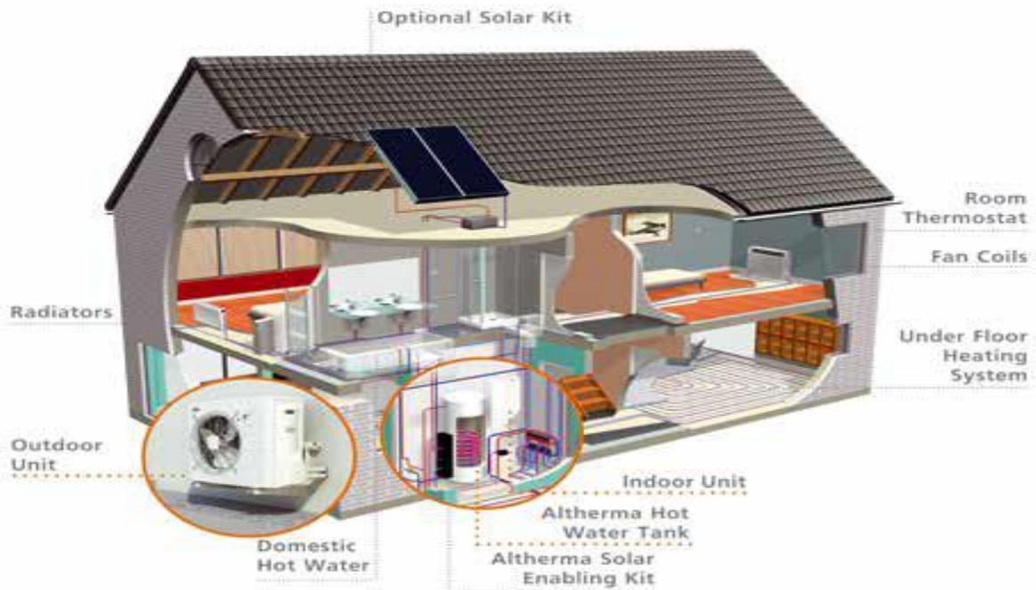
**How They Work** Air source heat pumps can extract latent heat from the outside air (even when the temperature outside is down to  $-20^{\circ}\text{C}$ ) and pump it inside to heat indoor spaces, making use of outside air as an infinitely renewable energy resource.
